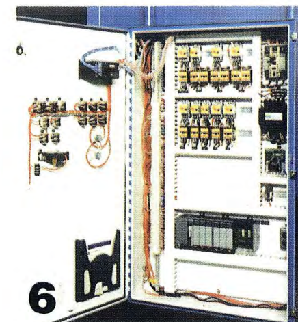
PLC (programmable logic controller) gives precise control of the palletizer and can be locked for safety.
