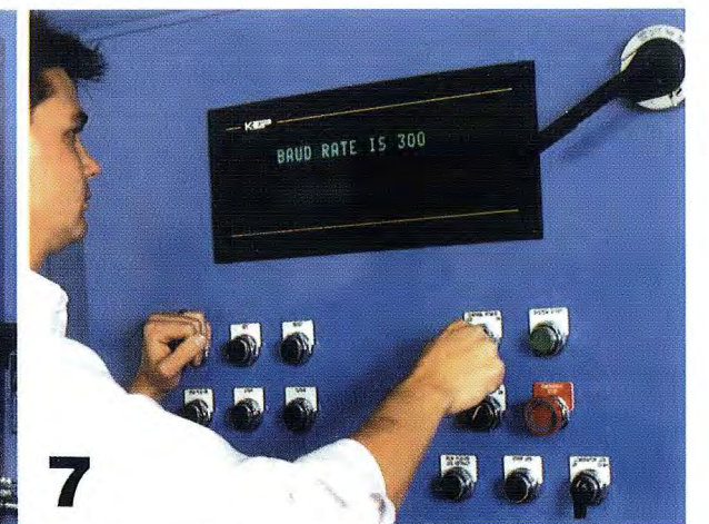
Diagnostic panel keeps tabs on the palletizing process, alerts the user of any abnormal situation, and provides diagnostic assistance with message display.
