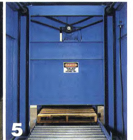
A four-corner, chain-driven pallet suspension system easily supports up to 4,000 pounds.
