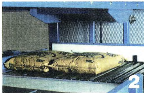
Overhead row pusher provides precise pallet-loading capability.
