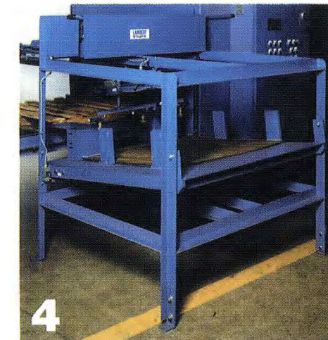
The optional slip sheet dispenser automatically places cardboard slip sheets on the pallet before loading.
