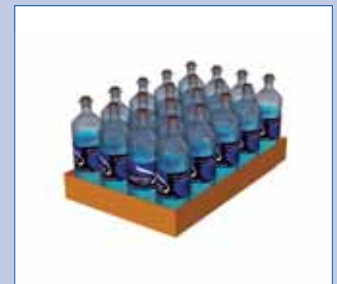
Hot melt glue is applied and the tray's (major) flaps are folded up, compressed & sealed.
