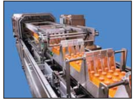
Infeed Section with Color Coded Spacers for Fast Changeovers
