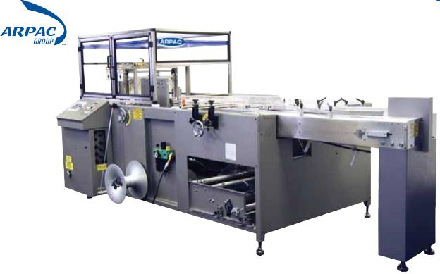
The TS37 side seal horizontal shrink wrapper is one of the most versatile packaging machines on the market today. Capable of wrapping up to 80 packages per minute, the continuous motion TS37 film folding system eliminates the need for multiple forming heads with its adjustable film former.
