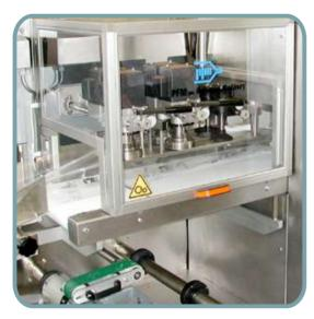
**Easy cleaning**: the construction concept is that of the "cantilevered" type, where the mechanical and electrical components are housed at the rear of the machine in separate and protected areas, while the sealing units and conveyor surfaces are housed at the front. The machine face is therefore free from obstacles and can easily be cleaned thus preventing production waste from coming into contact with mechanical and electrical parts.
