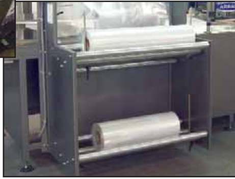
Side Mounted Dual Film Cradles for Easy Film Loading
