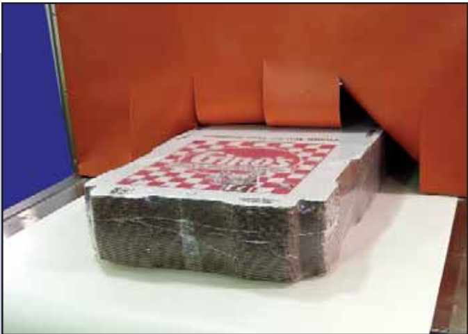
Wrapping Stacks of Corrugated Blanks
