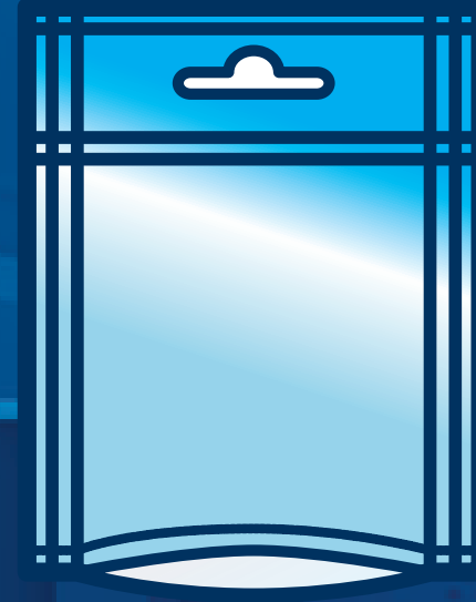
3 side seals stand-up bag with euro hole punch on vertical sealing bar and zip in line
