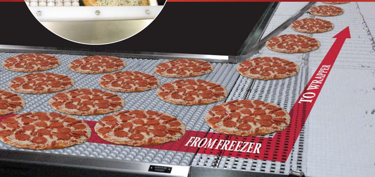
The low back pressure conveyor system gently accumulates and collates the frozen pizza products, without causing damage or shingling in a single rowing application.
