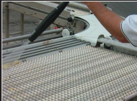
The stainless steel Easy Clean™ conveyor design integrated with the anti-microbial roller surface, inhibits the growth of bacteria, mold and other unwanted organisms, netting a cleaner conveyor system.
