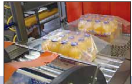
Transition Conveyor Section to Tunnel
