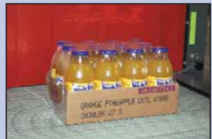
Finished Product Exits the Shrink Tunnel Through 3-Way Cooling Section
