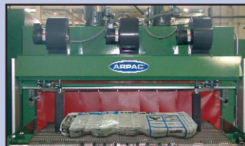
Shingles Exiting Shrink Tunnel
