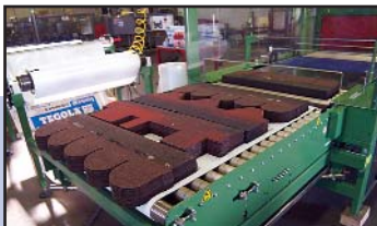
Shingles on Infeed Conveyor
