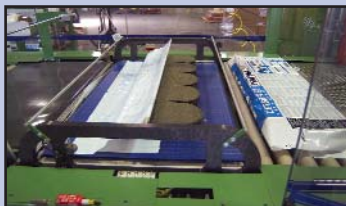
Shingles on the Overwrap Conveyor
