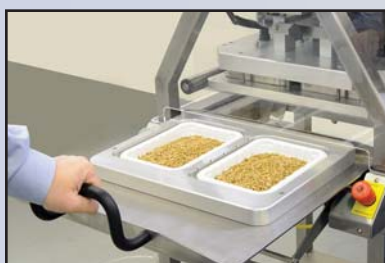
Product is loaded into the drawer and pushed into the sealing section.
