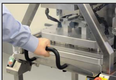
Seal head activates, flushing the product with desired gas mixture and sealing the tray.
