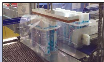
Bridge Plate for Small Product Transfer and Product Hold Down
