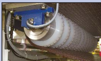
Motorized Pulleys Replace Greasy Chains
