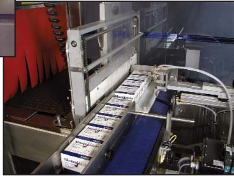
Right-Angle Infeed Conveyor with Intralox Belt
