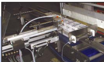
Main Ram Gently Pushes the Product into the Sealing Section
