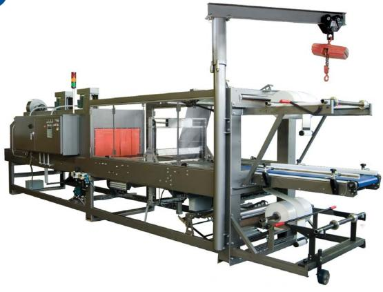
ARPAC's 65TW-28 tray wrapper is part of a dependable line of shrink packaging systems designed to meet the needs of today's high volume production lines. This compact and economical shrink wrapper is capable of wrapping up to 65 trays per minute, depending upon product size.
