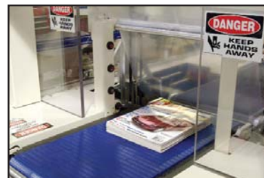
Automatic Product Height Detection for Random Sizes
