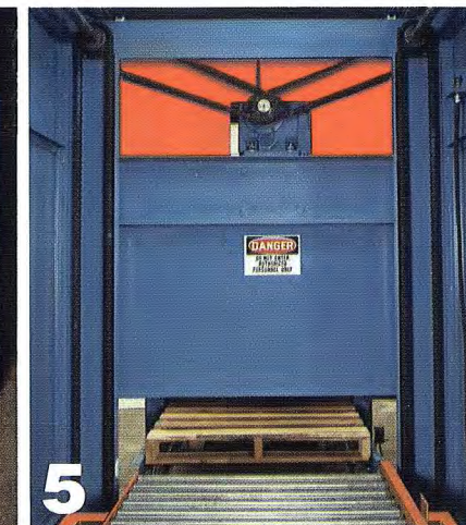
A four-corner, chain-driven pallet suspension system easily supports up to 4,000 pounds.
