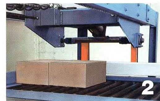
Overhead row pusher provides precise pallet-loading capability.
