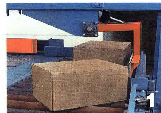
Rotator device precisely positions product to facilitate forming patterns.
