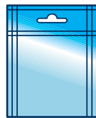
3 side seals bag (with euro hole punch on vertical sealing bar)
