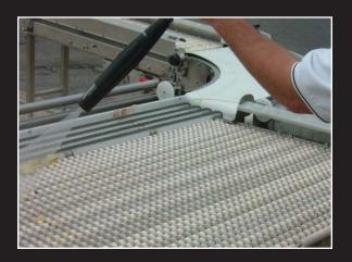
The stainless steel Easy Clean<sup>™</sup> conveyor design integrated with the anti-microbial roller surface, inhibits the growth of bacteria, mold and other unwanted organisms, netting a cleaner conveyor system.
