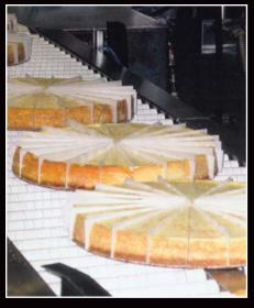
Shuttleworth's Herringbone conveyor automatically centers the most delicate products prior to wrapping without using guiderail or devices.
