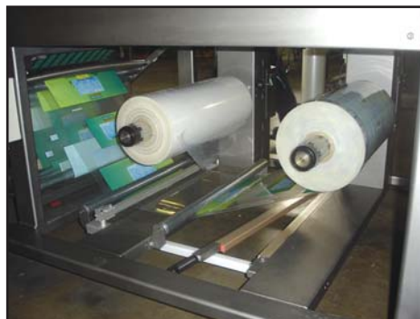
Inline Film Rack and Film Splicing Bar for Quick and Easy Film Changeover
