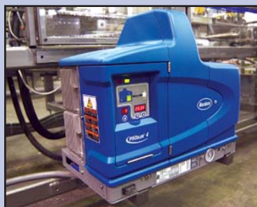
Standard Nordson ProBlue® Glue Unit
