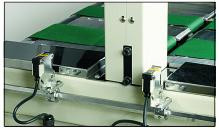
ADJUSTABLE PHOTO EYES FOR PRECISE STRAP PLACEMENT
