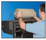
**Easy load film cradle** handles 30"CF width. Film threading from the front allows placement of machine close to a wall or in-line with conveyor system. Optional centerfolder available.
