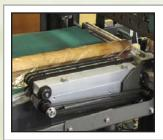
Proven side seal design works reliably and cleanly on polyolefins, PVC's and polyethylenes without buildup. It is the simplest, most reliable, time tested side sealer available on the market.
