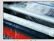
Adjustable Perforator with Brush Roller
