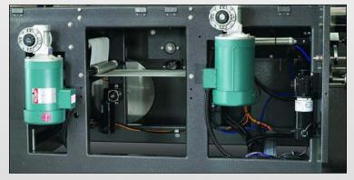
**Direct drives** eliminate chains, sprockets, take ups or need for maintenance or lubrication. **Cross seal** runs on 1" linear bearing shafts. Both features provide smooth high speed operation and reliability.
